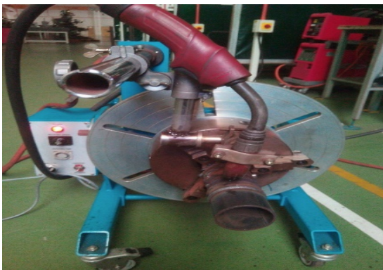
Figure 2. Welding Torch Transsynergic 4000 Attached To A Rotating Jig
