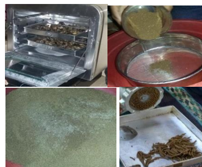
Figure 2. Snail flour production process
