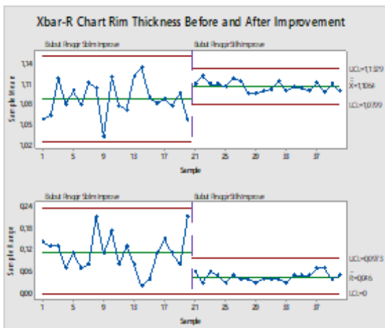
Figure 11. Control Charts of of the MU5-TJ Cartridge Case Rim Thickness before and after the Improvement
