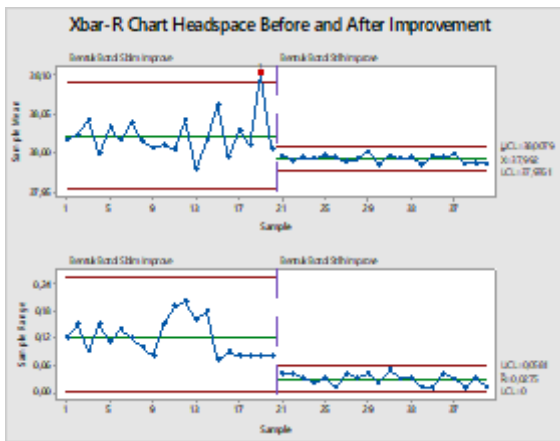
Figure 10. Process Capability of the MU5-TJ Cartridge Case Headspace before and after the Improvement
